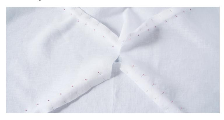
2. Stitch the pinned edges together 3/8 (1 cm), then trim the seam allowances down to 1/4 (6 mm) and serge/zigzag the raw edges together to prevent the fabric from fraying.
